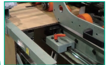
Glue flap will be folded automatically in the folding device. It is automatic suture start sheet of both you come to the set position.
